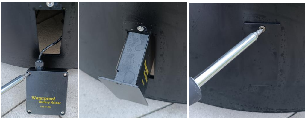
Fig. 9: Replacing the batteries in the container
