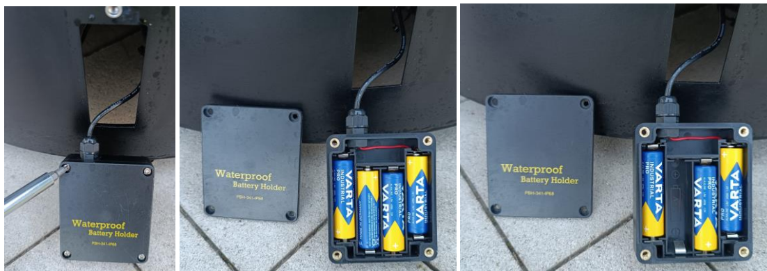
Fig. 9: Replacing the batteries in the container
