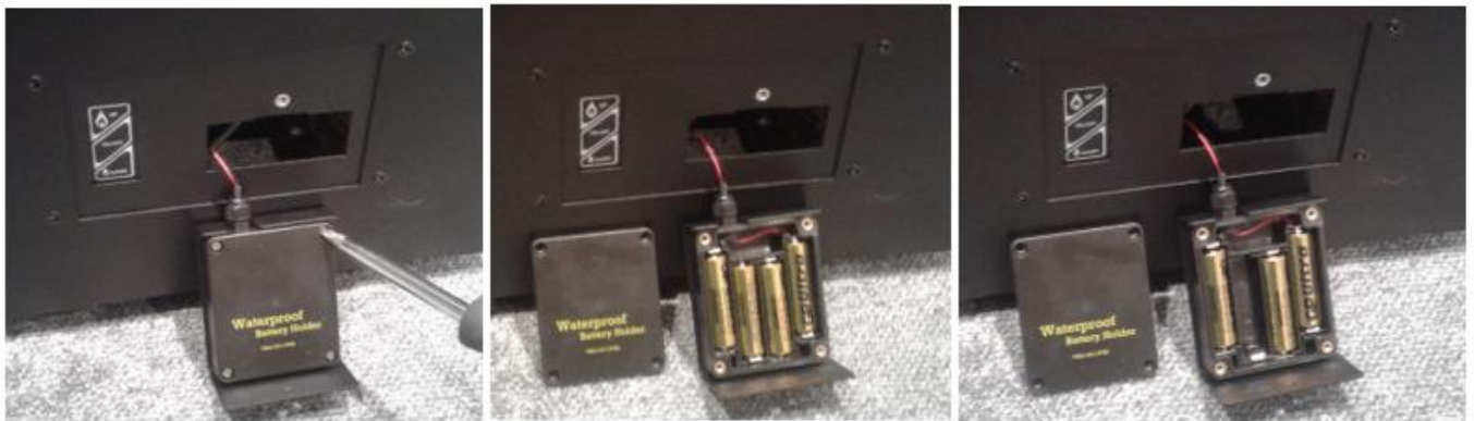
Fig. 10 – Replacing the batteries in the container
