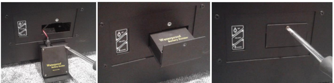
Fig. 11 – Putting back the battery box
