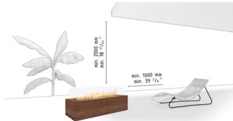
Fig. 1: Minimum distance to flammable materials
