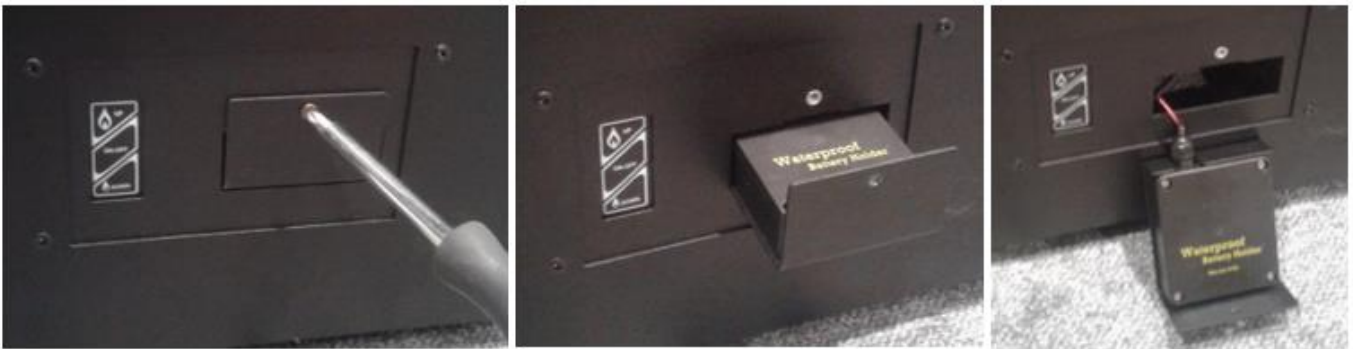
Fig. 9 – Removing of the battery container
