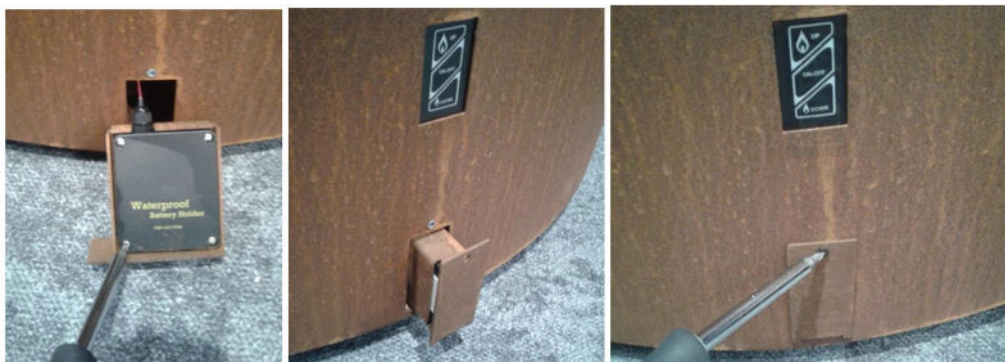
Fig. 9: Replacing the batteries in the container
