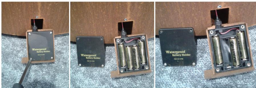
Fig. 9: Replacing the batteries in the container
